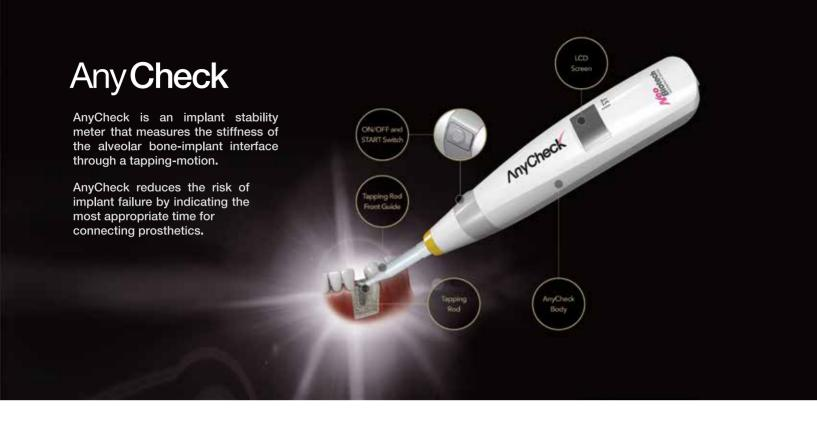
Measured value is similar to ISQ scale: above 60 - bridge recommended; above 70 - single case loading possible.
